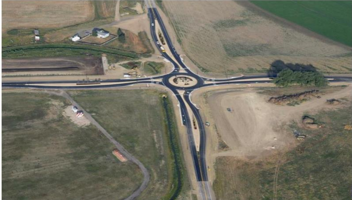
Figure 40 Rural Single-Lane Roundabout
