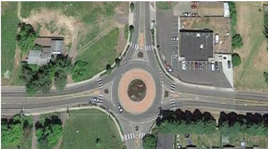
Figure 38 Urban Single Lane Roundabout
