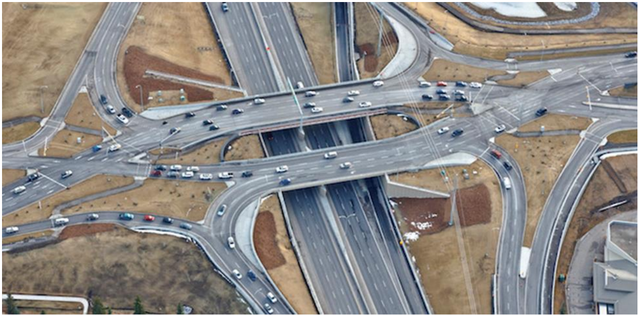
Figure 23 Diverging Diamond Interchange
